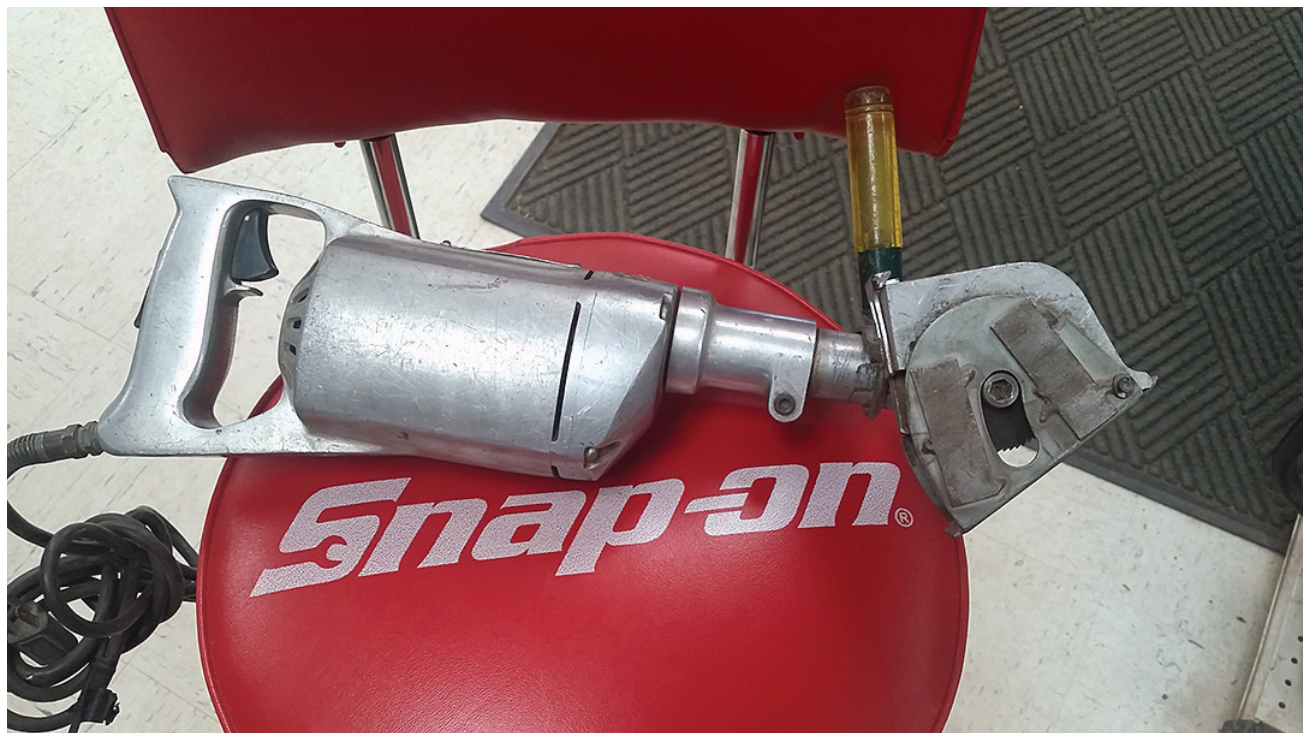
This mystery tool is a Kett Saw used to cut sheet metal without cutting into the interior framing, like cutting the skin of a metal door to install a window lite or a louver vent.
